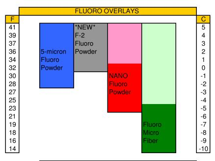
Fluoro Microfiber and NANO powder work at well higher temperatures. The darker colored area shows the preferred fluoro for that temperature range.
